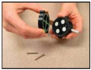
3. Liftoff the impaction plate to expose the base plate.
