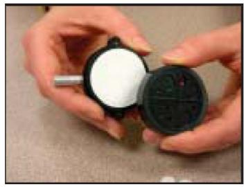
5. Use forceps to remove the collection filter and place it in an appropriate container for shipment to a laboratory.
