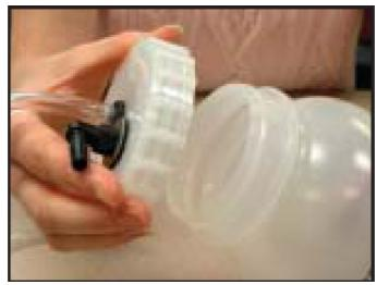
b. Using supplied adapter, attach soft tubing end to PPI outlet. Attach the rigid end of the adapter to Luer adapter in the center of the jar lid.
