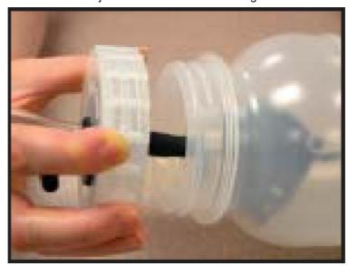
d. Attach center tubing on the outside of jar lid to pump inlet.
