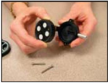
4. Using forceps, insert a 37-mm support pad and a 37-mm collection filter into the base plate.
