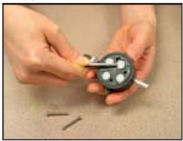
**Tip** Impaction substrates have a smooth/shiny side and a rough/dull side. For optimum particle capture efficiency, place substrate smooth/shiny side down in the impaction plate.
