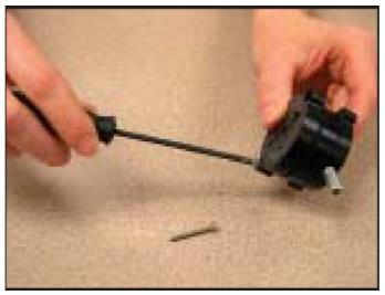
2. Liftoff inlet plate to expose impaction plate.
