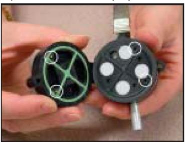
4. Grip impaction plate and inlet plate together and twist on base plate until screw holes are aligned.
