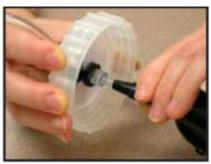
c. With PPI attached, place the lid on the jar and screw it down until tight.
