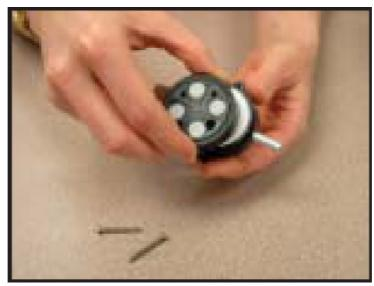
5. Replace and tighten two screws to secure the inlet plate to the base plate.
