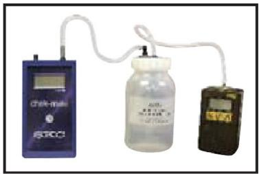
4. Disconnect tubing and remove calibration jar and calibrator when calibration is completed.
