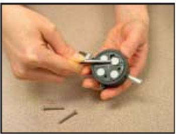
4. Liftoff the impaction plate to expose the base plate.
