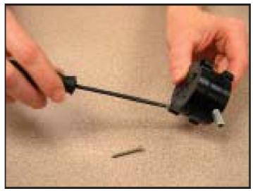
2. Liftoff the inlet plate to expose the impaction plate.
