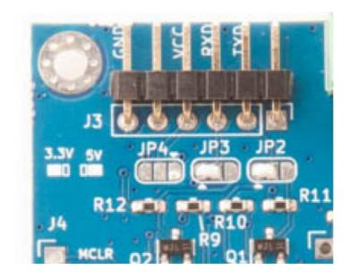
The UART connection is via J3. The UART voltage is selectable via JP2,3 Solder the bridges on the left for 3.3v. Solder the bridges on the right for Sv. Photo shown 3.3v been selected.
