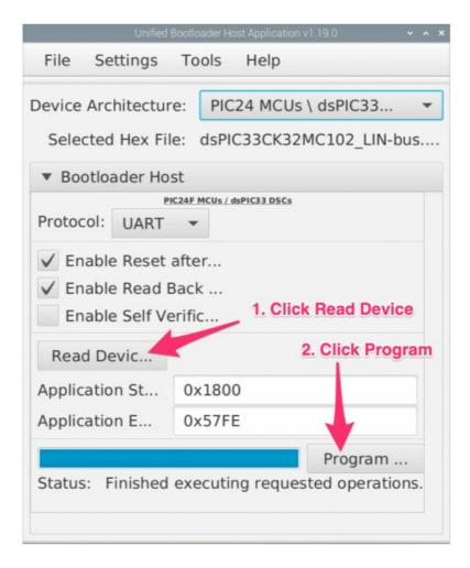
Check the Status shows Finished executing requested operations and no error shown. Remove jumper from board and power cycle.
