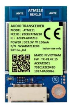
The hardware for the audio input (transmit) and audio output (receive) versions of the module is identical and only the firmware loaded onto the module determines its function. The distinction according to the module's function is to be identified by the module's label color and code name.
