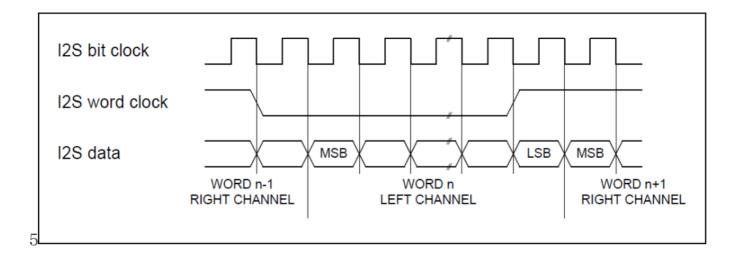
\*The timing specified for the rise and fall times represents the edge rates on the module itself. The rise and fall times of the I2S signals are determined by ESD/EMI mitigation components on the modules, as well as external loading, and will be higher than the specified numbers.
