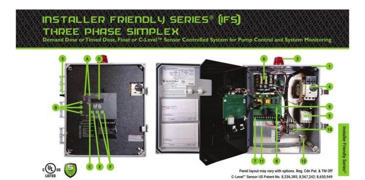
The IFS simplex control panel utilizes an innovative circuit board design to control one 208/240/480 VAC three phase pump in water and sewage applications. IFS panels feature an easy-to-use touch pad on inner door for programming and system monitoring. The panel configuration can be easily converted in the field to either a timed dose or demand dose. Available with the EZconnex® float system.
