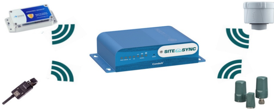
Figure 1. Lora Wan end devices with a Site Sync Lora Wan Conduit gateway.
