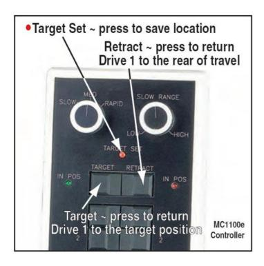
**Retract:** This is a black button that is located in the middle-right of the controller. This button only affects Drive No. 1.
