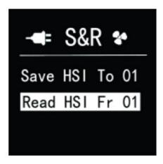
Long press the FN button to enter. CCT Mode, HSI Mode, RGB Mode and XY Mode support data storage. Rotate the knob to adjust Read/Save from 01 to 20. Hit the FN button, select Read/Save, rotate the button to select from 01 to 20 and hit the M button again to confirm.
