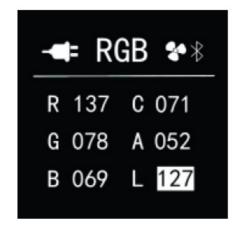
Hit the M button to enter RGB Mode. Press the FN button to select R/G/B/C/A/L. Rotate the knob to adjust from 0 to 255.
