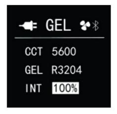
Hit the M button to enter GEL Mode. Press the FN button to select CCT, GEL and INT. Rotate the knob to select CCT 3200/5600, select Color GEL and adjust intensity from 0 to 100%. A total of 66 types of color gel. (22 for LEE and 44 for ROSCO)
