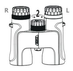
Open your left eye and close your right eye. Adjust the center focusing wheel (2) until the image is sharp.
