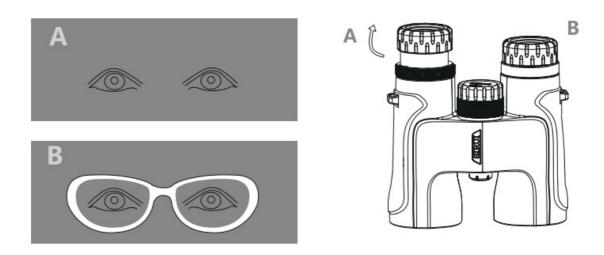
If you wear glasses, make sure the eye cup is fully retracted (B), and if not, make sure the eye cup is fully extended (A).
