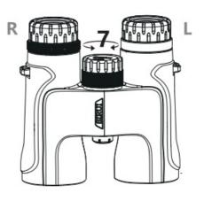
Open both your eyes and adjust the center focusing wheel (7) until the image is sharp.
