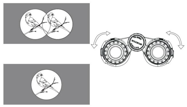
Hold the binoculars with both hands and move the tubes up and down until a single image is in the circle.
