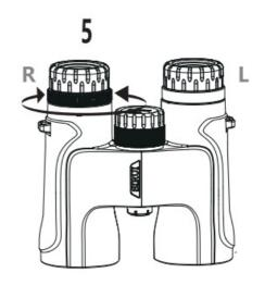
Open your right eye and close your left eye. Adjust the eyepiece focusing ring (5) until the image is sharp.
