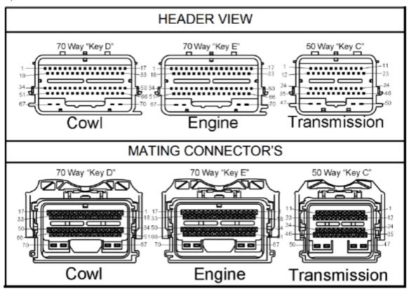
The Cortex EBC wiring harness can be connected to the PCM connectors as outlined in the following table (C = Cowl Connector, E= Engine Connector, T = Transmission Connector). RPM and vehicle speed signals are required for boost by gear applications.
