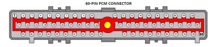
The Cortex EBC wiring harness can be connected to the 60-pin PCM connector as outlined in the following table. RPM and vehicle speed are required for boost-by-gear applications.
