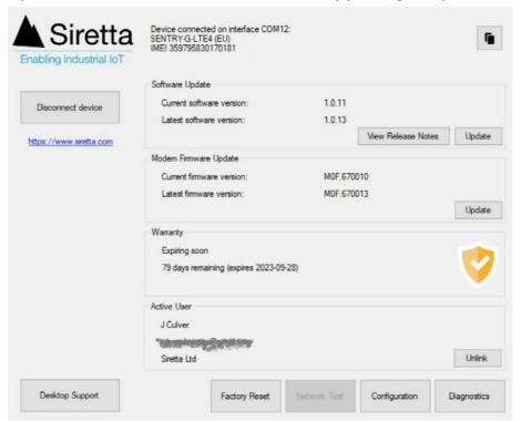
9. Power cycle the SENTRY after applying any update. If no updates are required, the update button will be inactive.
