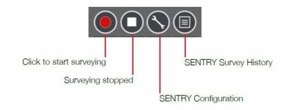
Click the survey configuration button to set up the cellular survey type required, its start conditions, and the required survey duration. Remember to click 'Update Device Information' to save the configuration. When the survey configuration has been set, click the survey button to start surveying.
