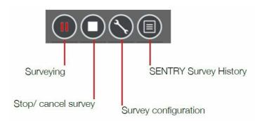
Then when surveying is in progress it changes to a red pause icon. To pause surveying, press the red pause button. To stop a survey immediately, press the stop icon. The survey button will change state to a timer while the SENTRY synchronises with the server. The view survey history button lists all surveys completed on the SENTRY.
