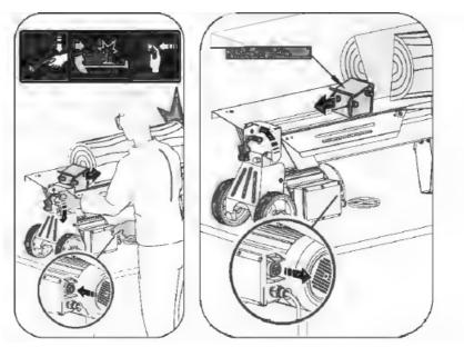
• Once the wood has been split, release the switch and hydraulic control lever, this will return the log pusher back to its starting position (above, right).
