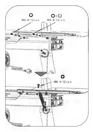
• Connect log support I (6) and log support 2 (7) with two M6x 12 screws and locknuts; Fully tighten to secure.
