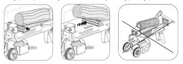
**CAUTION:** Do not try to knock the jammed log from the splitter with a hammer, using a hammer could damage the splitter or cause injury to the operator or those in the area.
