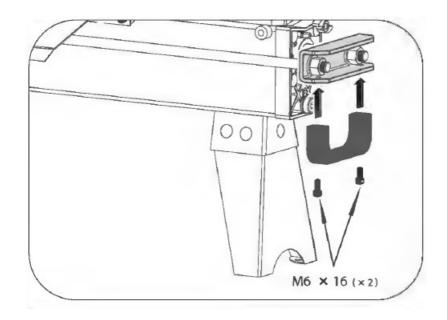
Mount the lifting handle to the bottom of the U bracket with two M6x 16 cap head bolts.
