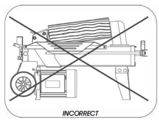
Set the log on the splitter so that the log will split in the direction of its growing grain; Do not place the log across the log splitter for splitting – it is dangerous and will cause serious damage to the machine. Do not attempt to split 2 logs at the same time!
