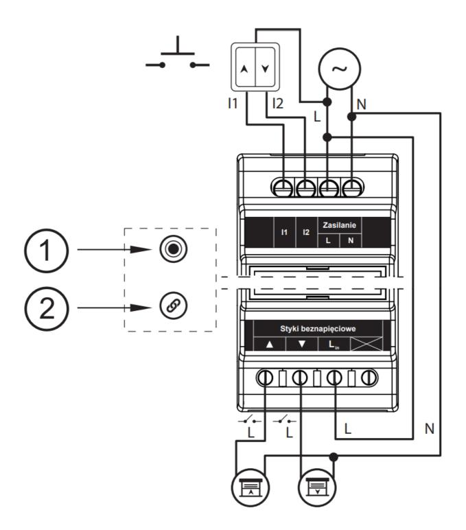
The PSZ-02 module is an electronic device equipped with 2 independent voltage-free relays enabling the user to control the roller shutter raising and lowering circuits. It can work with the monostable switches. It is designed to be mounted on a DIN rail. It communicates with the Sinum central device via a radio signal.
