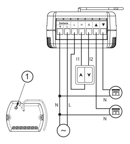
The PSZ-02 module is an electronic device equipped with 2 independent relays enabling the user to control the roller shutters with the use of a wall switch or an application. It can work with the monostable switches. It is intended to be mounted in an electrical box. It communicates with the Sinum central device via a radio signal.
