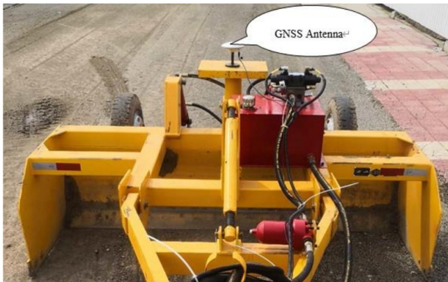
Figure 2.1 GNSS antenna installation
