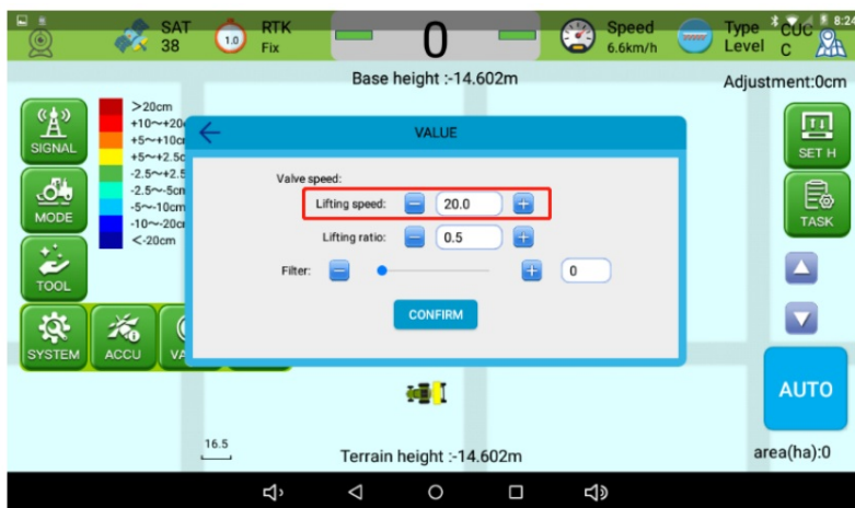
Figure 4.4 Adjust Sensitivity Value
