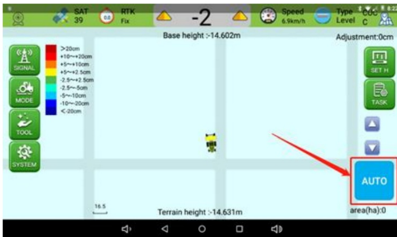
Figure 33 Start Automatic Leveling
