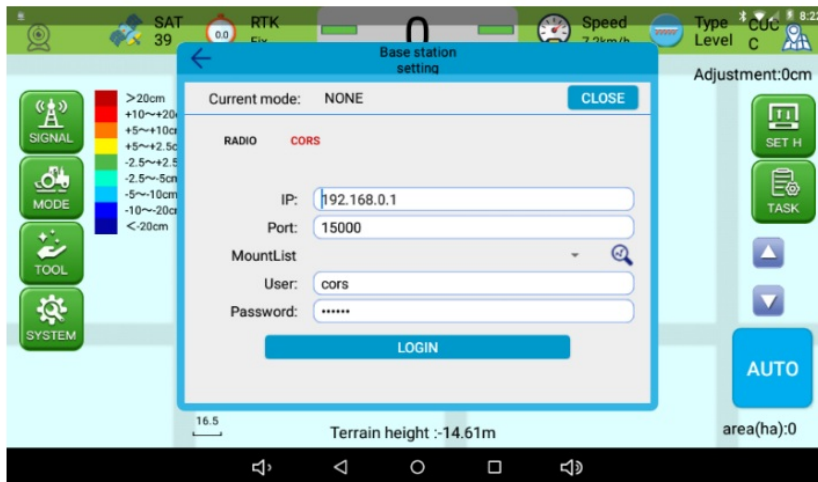
Figure 3.4 SIGNAL – Base Configuration Interface
