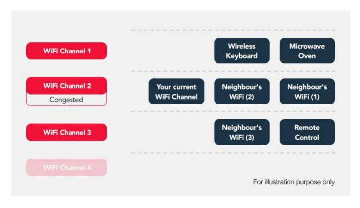
Channel congestion may result from signal transmitting devices and home electrical appliances interfering with the WiFi strength.
