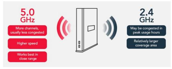
A dual-band wireless router is able to emit both 2.4GHz and 5GHz signals simultaneously. The 5GHz band offers
