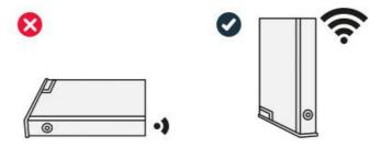
Do not stack your wireless router together with other electronic device or put it in small enclosed spaces to avoid overheating and damaging.
