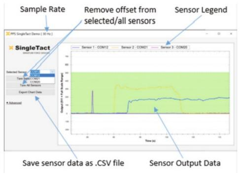
You are now ready to use your SingleTact system to make pressure and force measurements! **NOTE:** The GUI is scaled from 0 to 511, and so the measured force will be given by the following equation (unless otherwise stated on the GUI):
