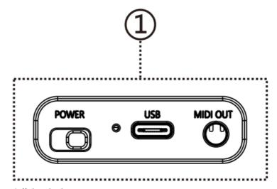
Power: Switch to turn on/off the device
