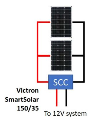
In this configuration, the panels have the capability of producing up to 870W, but the controller would adjust the
