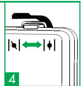
4 Move the choke to the CLOSED position.
