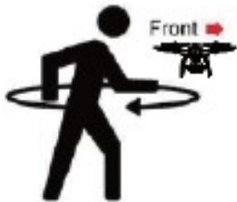
X-axis calibration, aircraft horizontal rotation
