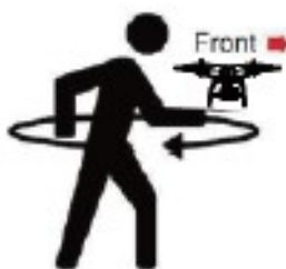
X-axis calibration, aircraft horizontal rotation
