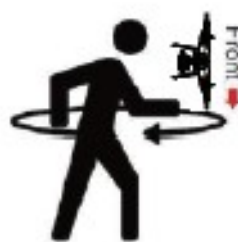
Y-axis calibration, aircraft vertical rotation
