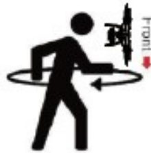
Y-axis calibration, aircraft vertical rotation
