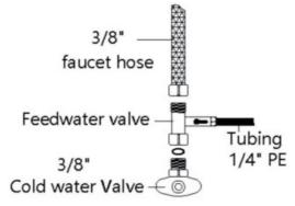
**Note:** Please check if the sealing ring is installed, or it may leakage. If the cold water valve outlet is 1/2", it can be connected via the following two fittings.
