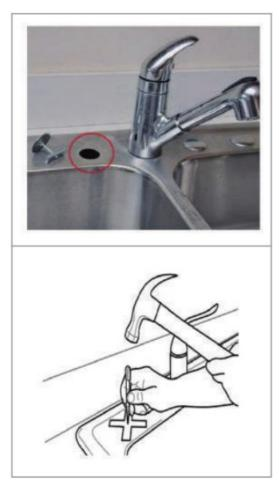
Using a hammer and center punch, mark the hole. Drill a pilot hole first, working up to "2" (12.5mm) drill bit. Insert the faucet through the hole with the top gasket in place and secure it with the locknut.
