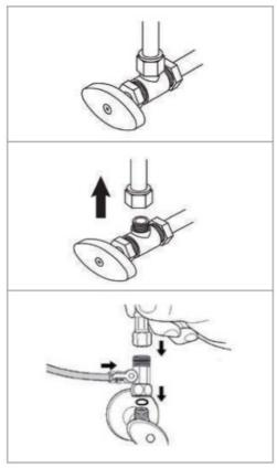
Remove the original connection from between the faucet and the cold water shut off valve under the sink. Connect the cold-water supply and feed water adapter valve.
