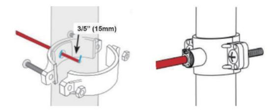
Step 5 – Connect Tubing (refer to page 17 for instructions on use of Quick Connect Fittings) Follow the instruction below to connect the SimPure® T1-400 Filtration System.
