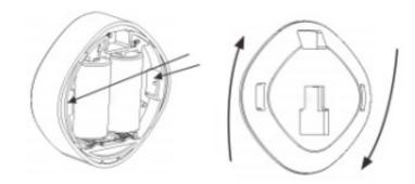
(2) Install the sensor's holder in desired location with crews or 3M glue.
