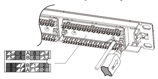
2. Punch down solid cable to each port until termination is completed.
