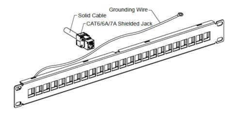
4. Expand the Foldable Cable Management Grip, hook the grips into fixture at both ends of the patch panel.
