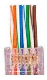
Push the plug down and over the cable jacket. (fig 1) The Simply45 ProSeries plug is designed to allow the cable to be inserted deeper into the plug than other brand RJ45 plugs. Notice in the picture (fig 2) that the cable jacket should come to the horizontal line underneath the plug. This is very important as you want to minimize the length of the untwisted wires. This design improves signal integrity and negates crosstalk interference
