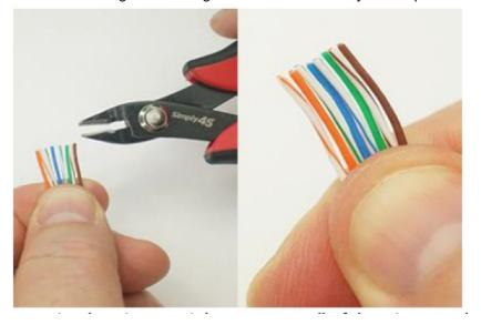
Using a flush cutter, trim the wires straight across so all of the wires are the same length. STEP 9
