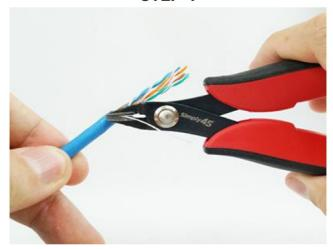
Trim off the "rip cord" at the cable jacket using Simply45 Flush Cutter.
