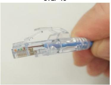
Then remove the terminated RJ45 plug from the crimping socket. Quickly inspect that all wires have been closely trimmed to the plug in the front.
