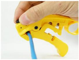
Using the Adjustable Cable Stripper, strip back the cable jacket about 1.5inches (3.8cm)
