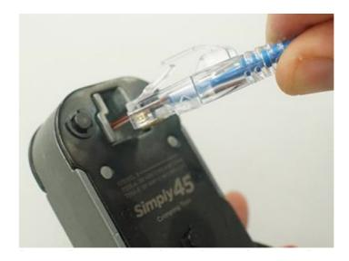
Insert the plug into the crimping socket on the Simply45 pass through crimper.
