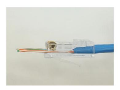
Push the plug as far down onto the cable until it stops inside the plug.
