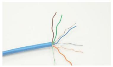
Separate each wire pair by untwisting.
