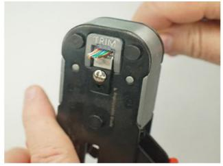
With one hand, firmly without stopping, compress the crimper handles all the way down in one steady non-stop motion.
