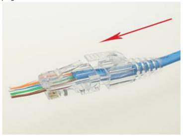
If using strain relief/boot, slide the boot up and into the back of the plug until the boot clip covers the top of the plug clip.
