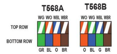
Align wires according to Termination Pattern either Type A or Type B.
