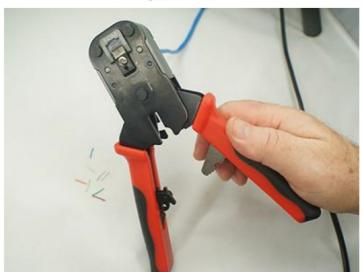
if the crimper handles do not release this means that you have not completed the crimping cycle. Simply squeeze the crimper handles further down until the crimper handles release.
