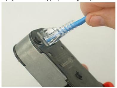
Make sure plug goes completely inside the crimping socket.
