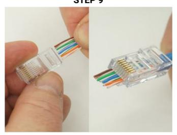
Hold the RJ45 plug upside down (strain relief clip facing down). Insert the wires into the back of the plug until they come out the front of the plug at least % inch (1.27cm).
