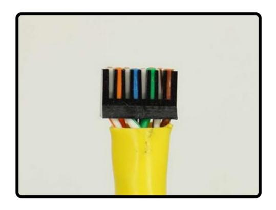
Then trim wires flush with the load bar using the Angled Flush Cutter (part: \$45-801 (https://simply45.com/shop/tools/cutters/s45-801-simply45-premium-5-flush-cutter-tool/)). Please be sure to trim wires properly. If wires are not trimmed close to the load bar, the load bar will not set properly over the Plug pins.
