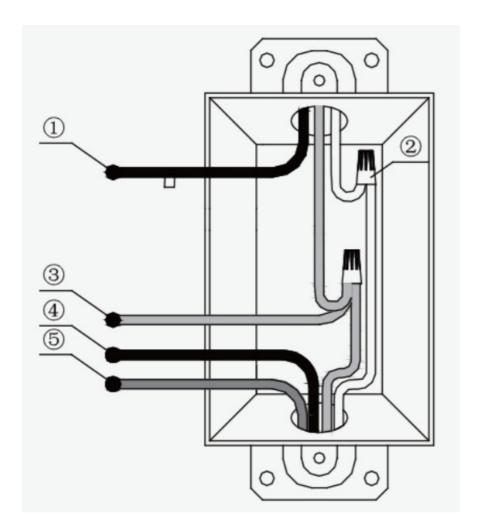
**Important:** Please note that for 3-way application, there is a power cord from the original switch be a different color (Black) or marked Common. Finding this power cord from both the dimmer's junction box and 3-way junction box ,then marking it as common (live or load).
