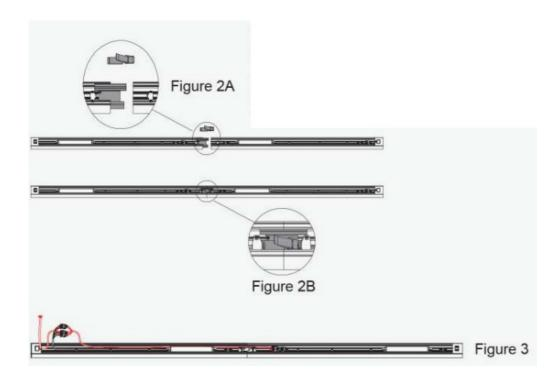
Pull the power cord of the fixture on the right to the fixture on the left inside of fixture body, and connect the wires one by one with quick connector. As shown in Figure 3.
