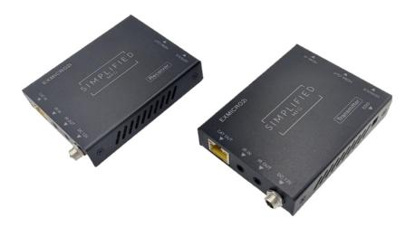
The EXMICR2i is the latest in the EXMICRO family. It is a HDMI 2.0b (18Gbps) over category cable extender that supports HDR/HDR10+. Other features include single ended power (either end), 50m distance at 4K (70m at 1080p), Bi-Directional 12V IR, HDMI loop out and EDID management. Small, efficient, and powerful.
