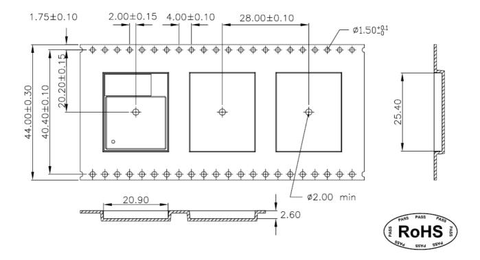
1. 10 sprocket hole pitch cumulative tolerance ±0.20.
