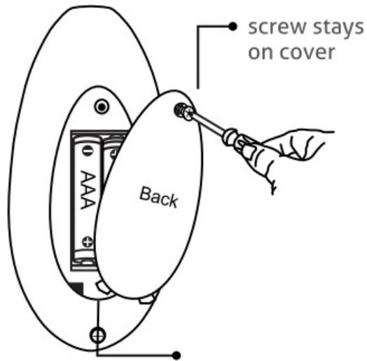
Insert two (2) AAA batteries, replace the backplate and re-tighten the screw. Be careful not to over tighten the screw.
