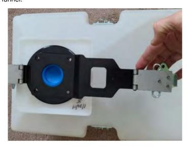
Install Quick-Attach Latch
