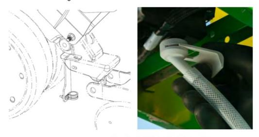
Install Quick-Attach Latch
