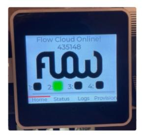
IT IS EXTREMELY IMPORTANT TO MAKE SURE YOU HAVE THE POWER PACK PLUGGED INTO THE FLOW DEVICE. The flow device has a battery back up which allows you to power up the device and configure it without plugging the power cord into the device. If you do not plug the power pack into the device, the battery will drain within a couple of hours and then power down. It is essential to check this before the completion of the installation.
