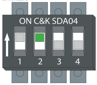
switch 2 → ON – Bluetooth communication enabled OFF – Bluetooth communication disabled
