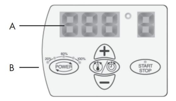
A) The main display shows the selected time or temperature for heating.
