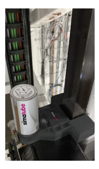
The special brush enables lubricant to be applied evenly. The lubricant is conveyed from the simalube lubricant dispenser to the brush and thus transferred to the guide. The brush touches the guide on three sides, is spring-loaded and automatically adapts to the rail. The simalube is driven by a gas producing dry cell. The amount of lubricant can be continuously adjusted directly on the dispenser with a running time of 1-12 months.
