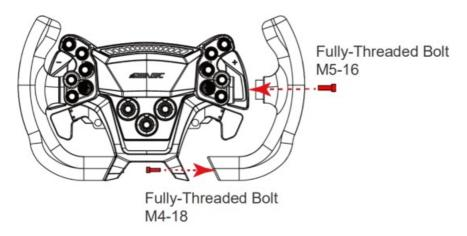
Position the handle grip on the corresponding area of the steering wheel, then install one M5-16 fullthread socket cap screw on each side. Additionally, install one M4-18 full-thread socket cap screw on each side at the bottom to complete the installation.
