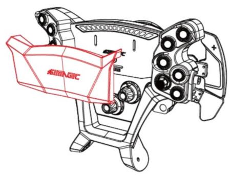
2. Install the magnetic connector for the screen, aligning it with the screw holes on the quick-release adapter plate.
