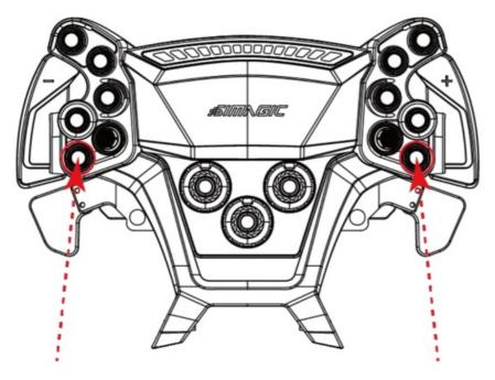
Press and hold the two indicated buttons simultaneously for 5 seconds to reset the wheel back to factory default settings.
