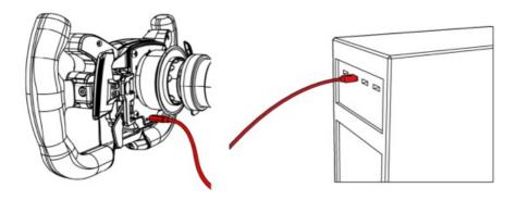
If there's no response when using the auto pairing mode, attach the included USB Type-C cable from the socket at the back of the wheel to the socket on the PC to manually sync the frequency (Please unplug the cable before driving in wireless mode)
