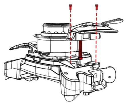
Remove the two screws and disconnect the terminal to replace the paddle shifter set.
