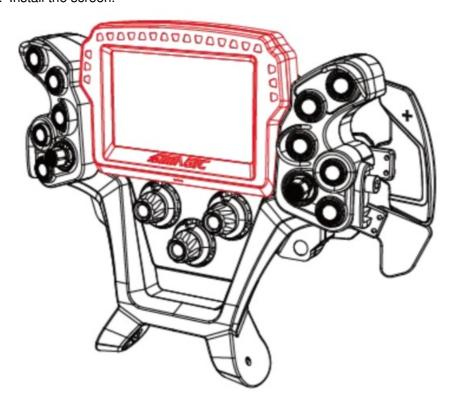
When the Zeus series steering wheel is connected to the Alpha Mini, Alpha, or Alpha U base, it can be used wirelessly via the quick-release base connection if no magnetic screen is attached. If you wish to attach a magnetic screen, an additional Maglink device is required to ensure proper screen functionality.
