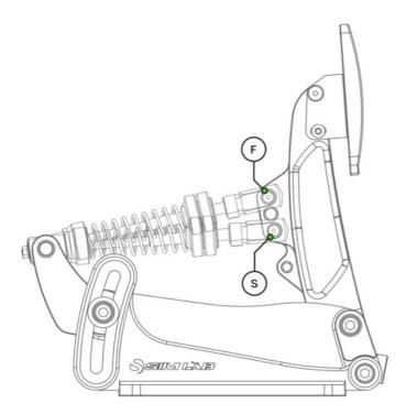
**Note:** by the nature of the position of the clevis fork so low on the pedal arm, travel might be mechanically limited. Please do check the travel manually (meaning literally, by hand) to see if you need to decrease travel using the travel adjustment knobs,to prevent the clevis fork interfering with the flange on the pedal arm. When it does, please reduce maximum travel until you have about 3-4mm between the flat base of the clevis fork and the pedal arm flange.
