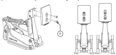
As mentioned, it is also possible to change the angle of the pedal face. Begin by loosening the top (T) (countersunk) bolts, but do not remove them. Temporarily remove the bottom (B) bolts and now the bracket can rotate freely. The bracket comes with a preset slot for different angles you can choose from. Choose your angle and fix it in place using the two bottom bolts (B). When happy, tighten the upper two (T) bolts again
