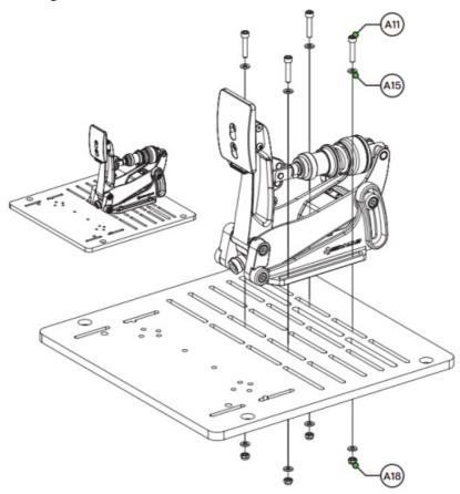
For normal pedal decks, the same hardware applies. The bolts will stick out a bit, that is okay
