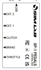
All pedals are plugged into the control box the same way. All inputs are labeled, for reference, here is top-down drawing with the same information as found on the box.
