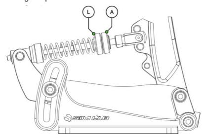
The same principle applies to the maximum travel of the pedal. On the bottom of the pedal arm you will find two blue knobs as well. The inner one is the travel locking knob (L), the outer one is the travel adjustment knob (A). Turning the adjustment knob clockwise results in less travel, turning the adjustment knob anti-clockwise results in more travel. By default, the pedal has been setup to provide a middle of the road range of travel but you are free to experiment.
