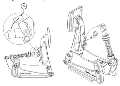
Release any tension from the spring by loosening any adjustment knob(s) before trying to remove the spring bolt.
