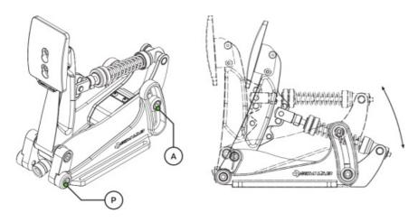
The angle of the pedal arm in relation to your cockpit can be changed by adjusting the pedal base. Simply loosen four bolts, start with the two (P) where the arm pivots around. After those are loose, loosen the two (A) in the arcs. Now you should be able to rotate the entire pedal as a whole while the base remains fixed in place. Tighten all bolts again after you have found your preferred position and you are good to go.
