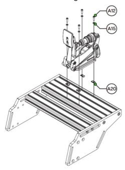
The example on the right shows the pedals mounted to the bigger of the two profiles to allow for a heel plate to be fitted on the smaller profile. This of course depends on your preference.
