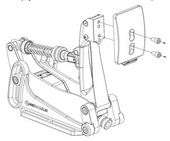
Add the foot support between the pedal arm and pedal face. Use the new bolts supplied (A2) to secure all parts.
