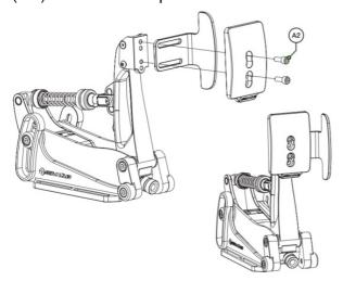
Loosen the bolts (A2) to be able to adjust the foot support and tighten when happy with your setting. The part is symmetrical is not limited to only being used on the throttle pedal.
