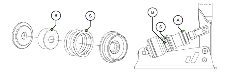
On the next pages we will show you how easy it is to disconnect the brakestack to add the preload buffer (B) and/or change elastomers.
