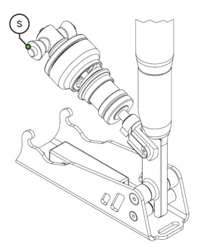
Depending on the spring you installed, the previous description can be hard to do. To counter that you can also choose to loosen the 'Spring Pin' (S) and rotate the entire brake stack away from the handbrake in the following way. Again, make sure you loosen the blue adjustment and locking knobs and thread them all the way up to the clevis fork (F).
