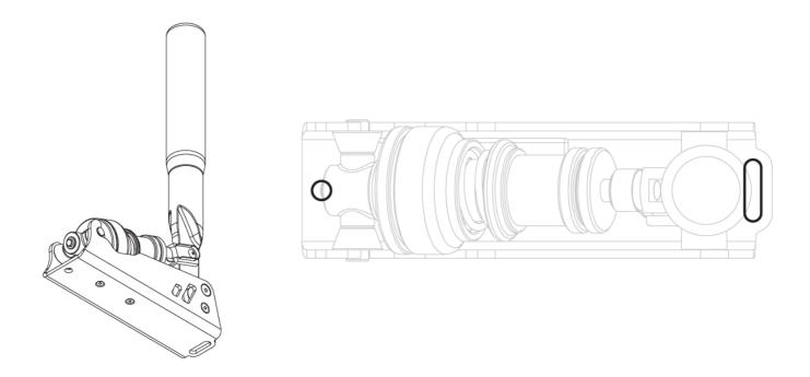
Using the handbrake mount purchased seperately, the handbrake can be mounted to the side of a shifter. The mount is compatible with our existing shifter mounting bracket and allows for roughly 20 degrees of outward rotation.
