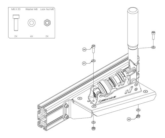
The maximum angle the handbrake can be positioned at is about 20 degrees. With the two shorter slots, you can make sure to clear a big h-shifter
