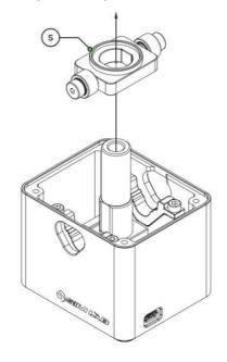
If you have trouble re installing the roller platform onto the main pivot, maybe rotate it 180 degrees. This is normal, the system is designed to have as little play as possible to work and feel as intended. Please make sure, the black nylon part is pointing upwards when installed. This is the seat (S) for the spring.
