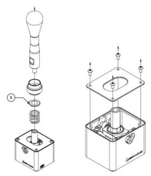
Next part to remove is the roller platform. This is a very important assembled part, so please take care of it. Simply pull free of the main pivot to remove it. This is a close fitting part, which contributes greatly to the precise feel of the shifter.
