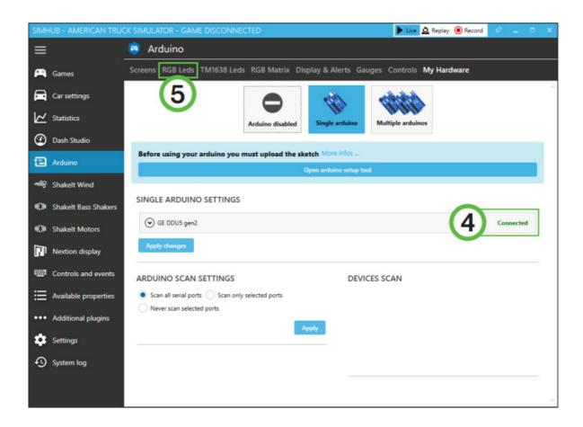
After we have confirmed the connection, press 'RGB Leds' (5) in the top row of options.
