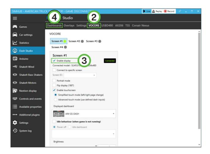
In the 'Screen #1' section, check 'Enable display' (3). The 'Connected' indicator will appear on its right-hand side. When the screen is connected, go back to 'Dashboards' (4).
