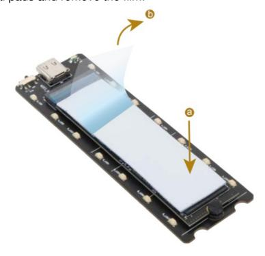
• Align the aluminium plate with the mounting holes, then lightly press to ensure a tight fit.
