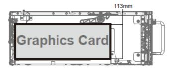
2. Height limitation with expansion card clip buckle removed
