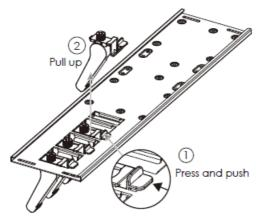
5. Adjust the position of the expansion card retainer according to the required height of the interface card, then tighten the screw
