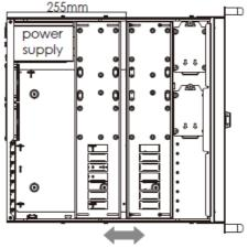
3. The maximum length limitation for graphics cards, front panel case fans, and the radiator is 424mm
