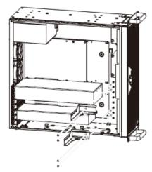
3. Once the graphics card bracket is pushed into position, tighten the thumb screw and then the graphics card screw.
