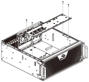
2. Expansion card retainer position shift (It is recommended to avoid the position of the expansion card connectors, and make sure the length of the PSU will not interfere.)
