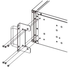
2. Remove the handlebars on both sides
