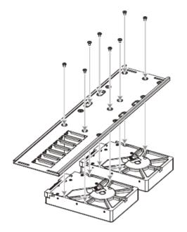
4. Install 3 x 2.5" SSD on the expansion card retainer
