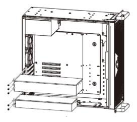
2. Install Nvidia 30 series graphics cards bracket (slightly tighten the screws, and reserve space for the bracket to slide left and right)
