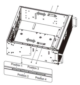
3. Install 2 x 3.5" HDD on the expansion card retainer
