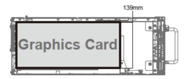
3. Height limitation with expansion card retainer removed
