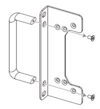
3. Install the handlebar onto the flat handlebar bracket
