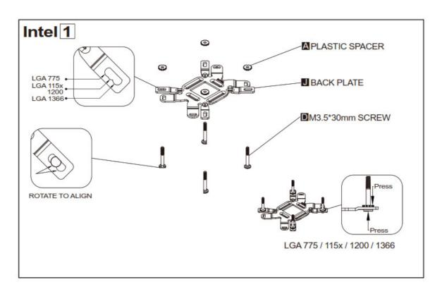
Make sure you are using the correct side of the backplate for your motherboard and insert the screw into the correct holes based on the CPU socket you use
