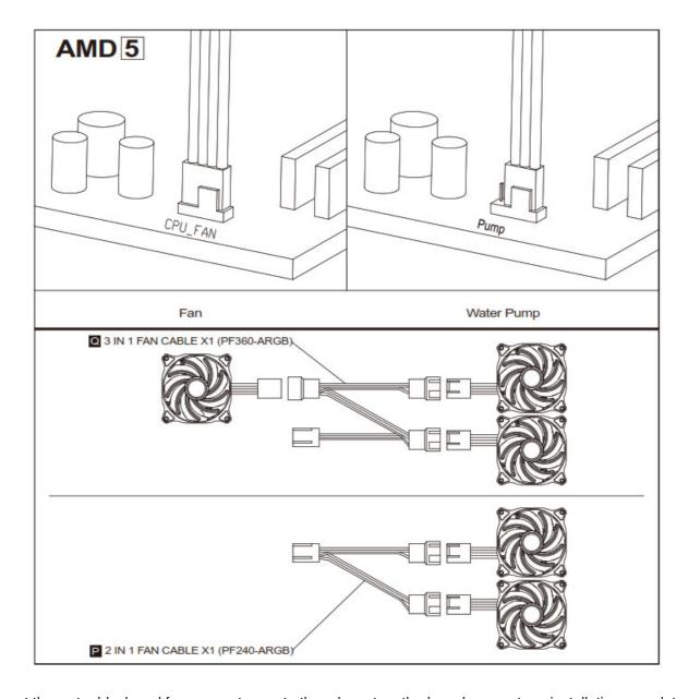
Connect the water block and fan connectors onto the relevant motherboard connectors, installation complete
