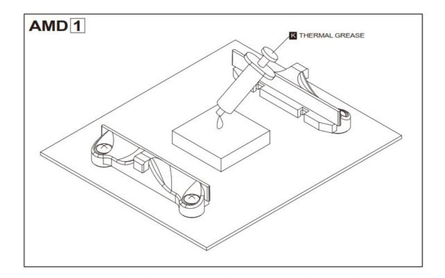
Please clean the surface of CPU before applying thermal grease evenly on the CPU
