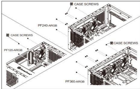
Secure the fan together with the radiator onto the chassis
