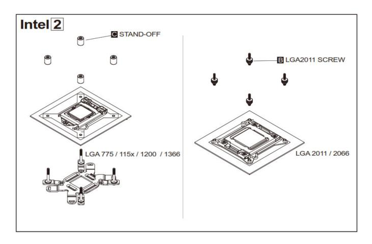
Install the backplate assembly onto the motherboard and slip on the screw standoffs \*Mount LGA2011 and INTEL clips and tighten the nuts
