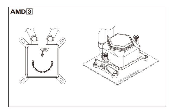
Remove the film from the waterblock's base and place it on the CPU
