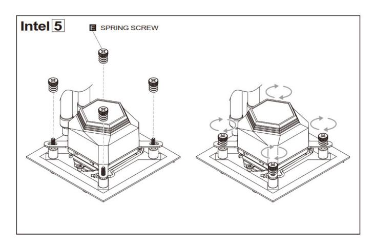
Secure the spring screws onto the screws with a screwdriver
