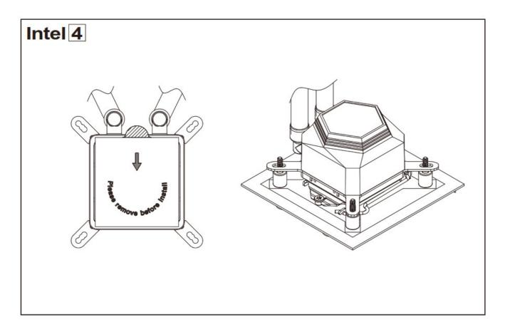
Remove the film from the waterblock's base and place it on the CPU
