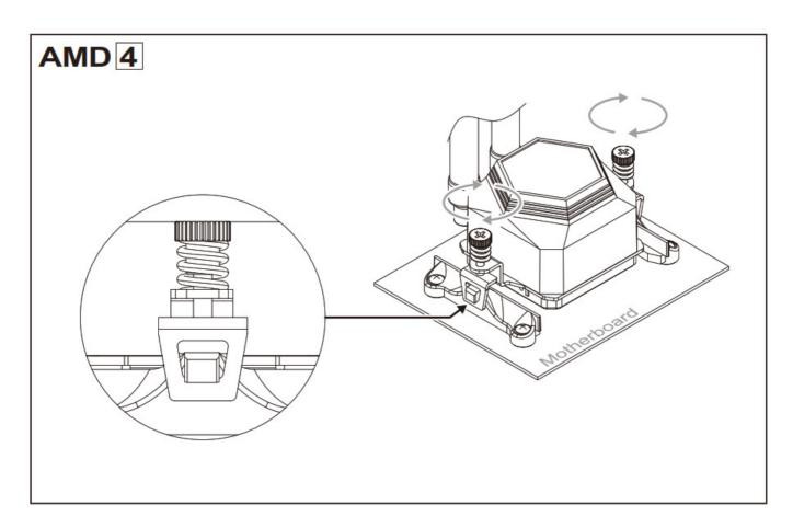
Hook the clip onto the motherboard's cooler retention bracket
