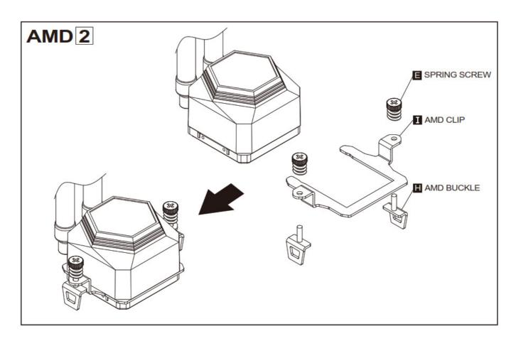
Remove the INTEL clips and install the AMD clips
