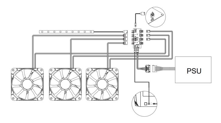
Restart lighting: After connecting the LED button of the chassis to the controller, long press or click once on the LED button to restart lighting.
