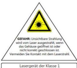
The device works with an invisible laser scanner. To prevent danger, the device may only be opened by a specialist.
