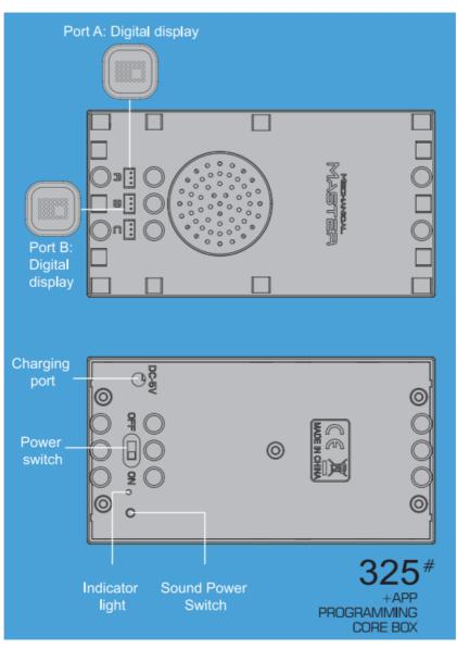
Charger block(Not Included) Power supply:5V 1-2A (DO NOT suggest power supply higher than this)
